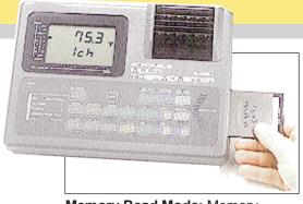
Memory Read Mode: Memory Data Selection: By specifying memory label and displaying data of selected channel (display by elapsed time also supported)
